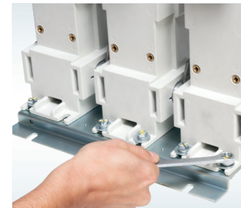
Figure 68: Type 12SVC400 (400 A) contactor - unbolting pole assembly from base
