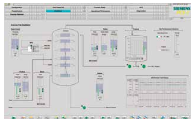
PCS 7 APG Distillation Column
