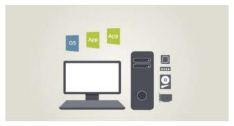
Virtualization decouples a computer's **operating system** and **application software** from its **hardware**
