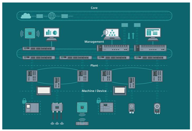
Connecting the IT and OT networks, with their different requirements, can be accomplished by starting with a defined backbone for the industrial side. The machine and plant-floor aggregation levels are in production scope. The backbone aggregation level is still an integral part of the production scope but aligned with IT in regard to the interface.
