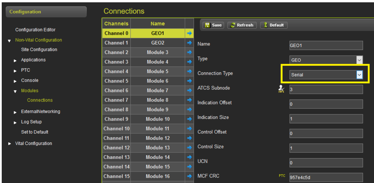
Figure 4-24 Setting the GEO Connection Type
