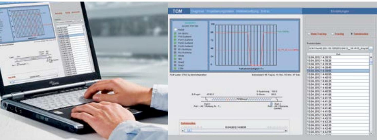
Using a standard PC, an integrated website can be opened in various languages (English, German, Spanish, etc.) via a web browser. This website allows quick access to the Clearguard TCM 100 modules in the network of the track vacancy detection system.
