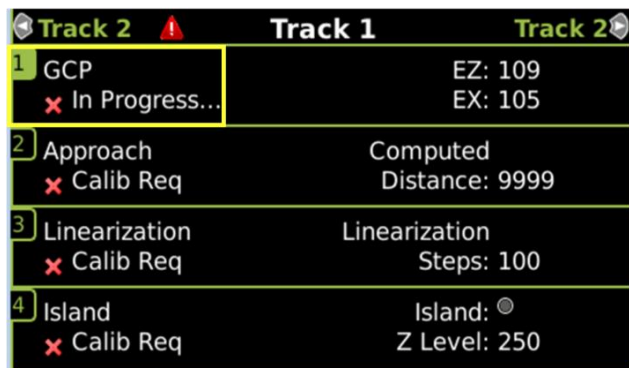
Figure 6 Calibration In Progress and Complete
