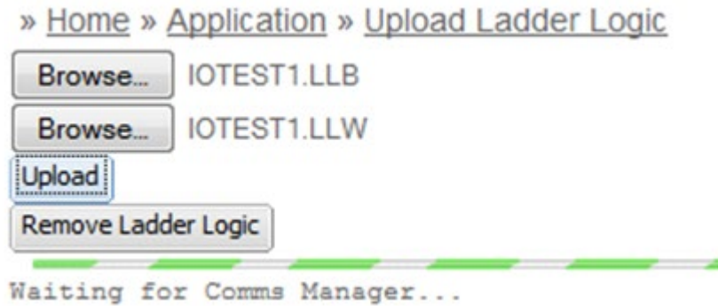
Figure 4-104 Upload Ladder Logic Files – Uploading in Progress
