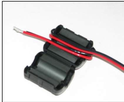
Figure 3-6 EMI Filter Installation (showing wire loops)
