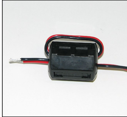
Figure 3-7 EMI Filter Installed
