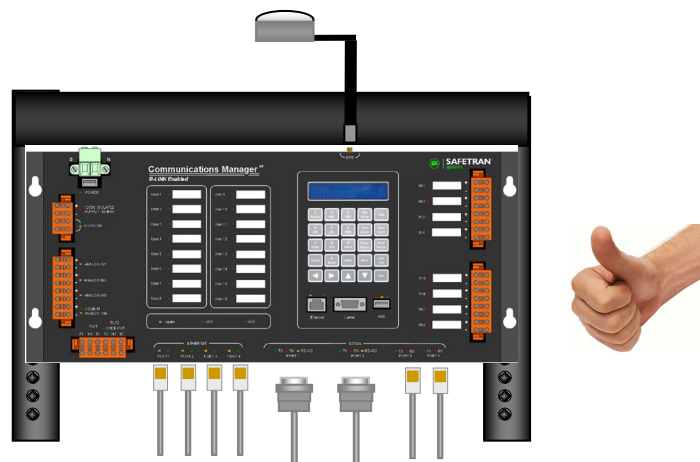
Figure 7-5 Re-install Communications Manager – Returning System On-Line
