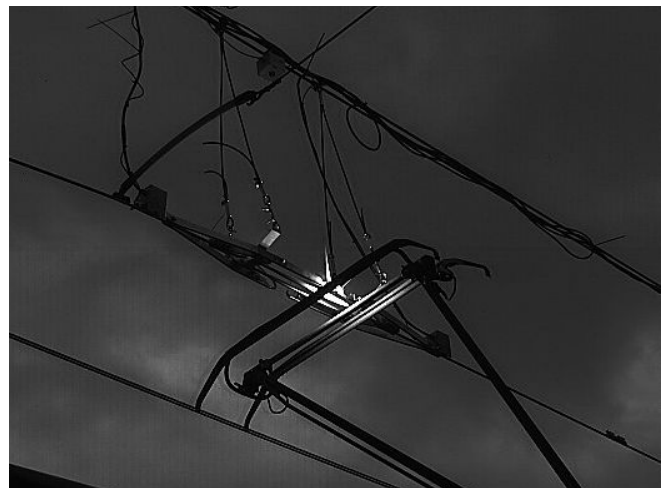
② Time 0 ms: Demolition arc is ignited
