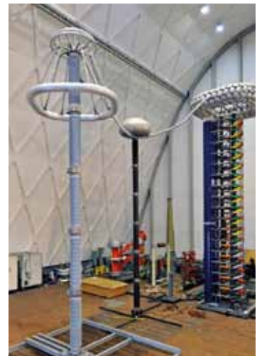
UHV arrester prepared for testing in the HV test laboratory
