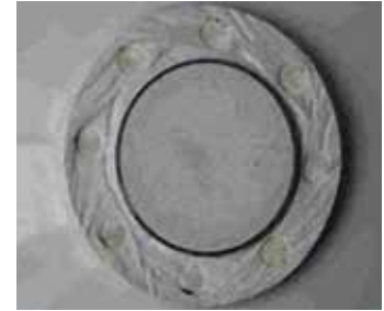
Horizontal cut of a cage design arrester
