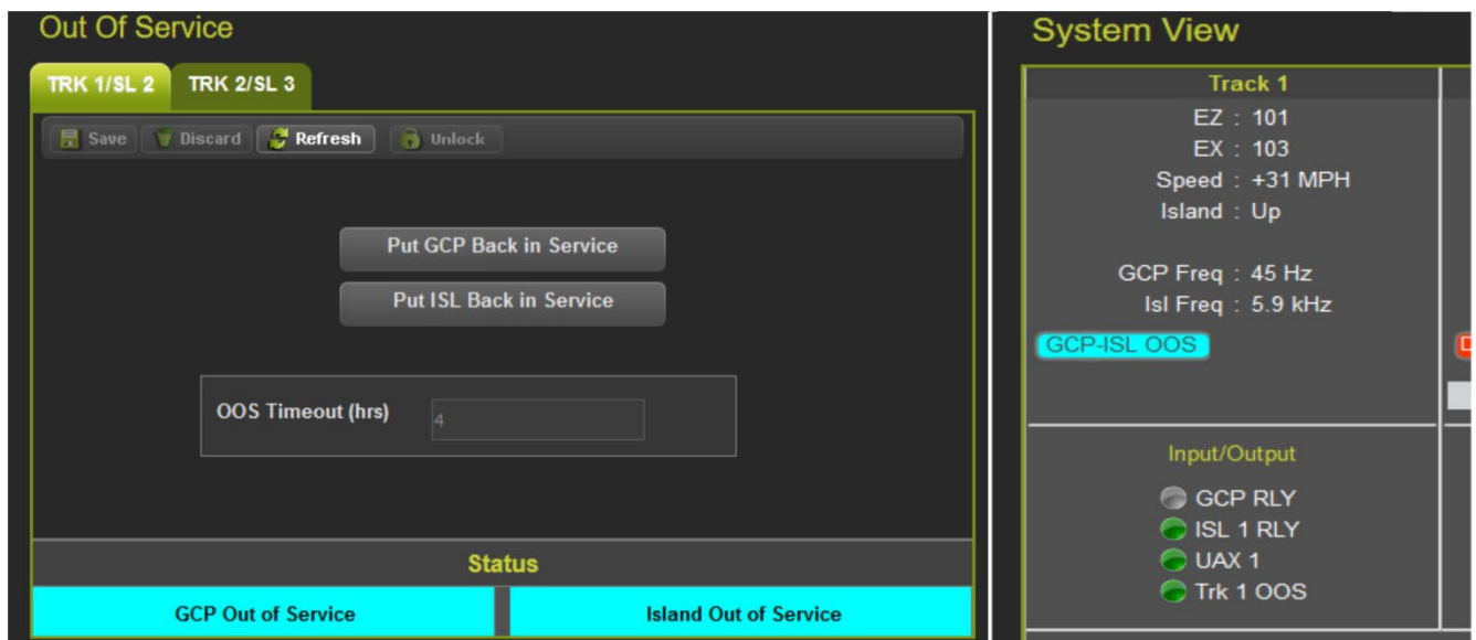
Figure 4-6: Island Out of Service Indications on WebUI
