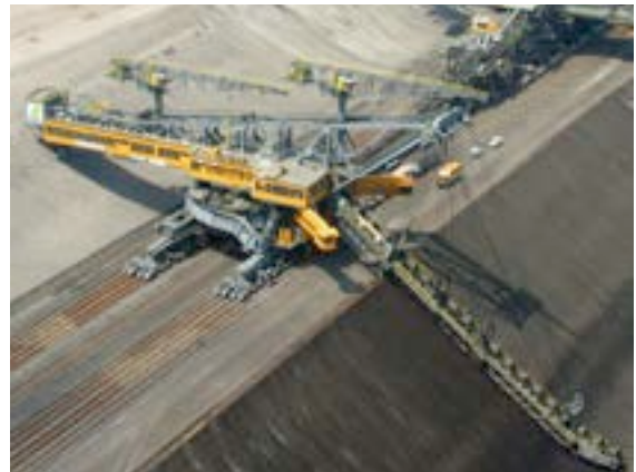
Bucket Chain Excavator
