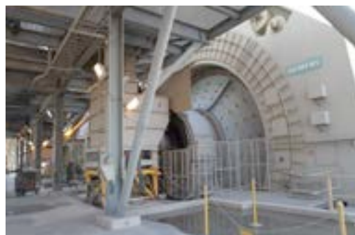
Highly efficient at variable speed – gearless AC drives for grinding mills
