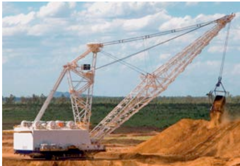
Highly efficient Caterpillar 8750 conventional dragline in operation
