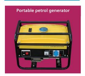
Portable petrol generators consist of two main components. Firstly there is a petrol engine; this is a type of internal combustion engine in which petrol vapour is mixed with air and ignited inside a cylinder. The rapid combustion forces the piston down the cylinder, turning the crankshaft. The energy has been transferred from the fuel to the crankshaft which is now spinning.
