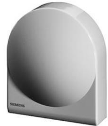
QAC22 Aussentemperatursensor Ni1000 -50..+70°C
