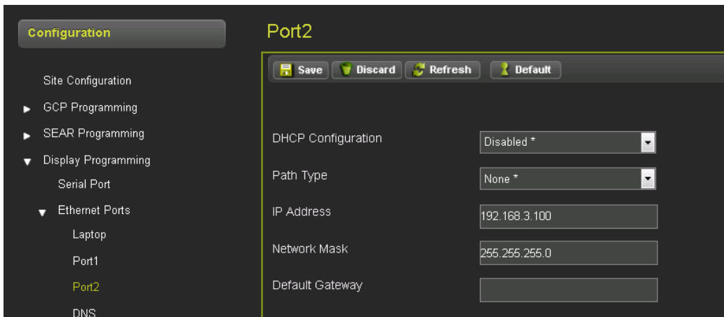
Figure 3-162 Display Programming: Port 2 Ethernet Port
