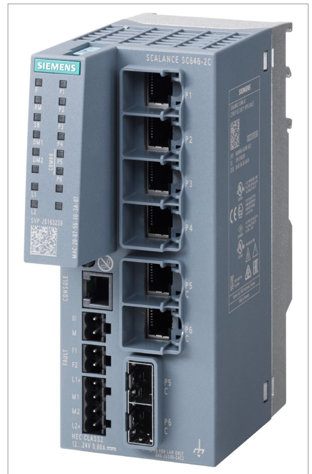
Figure 3. The SCALANCE SC646-2C Industrial Security Appliance
