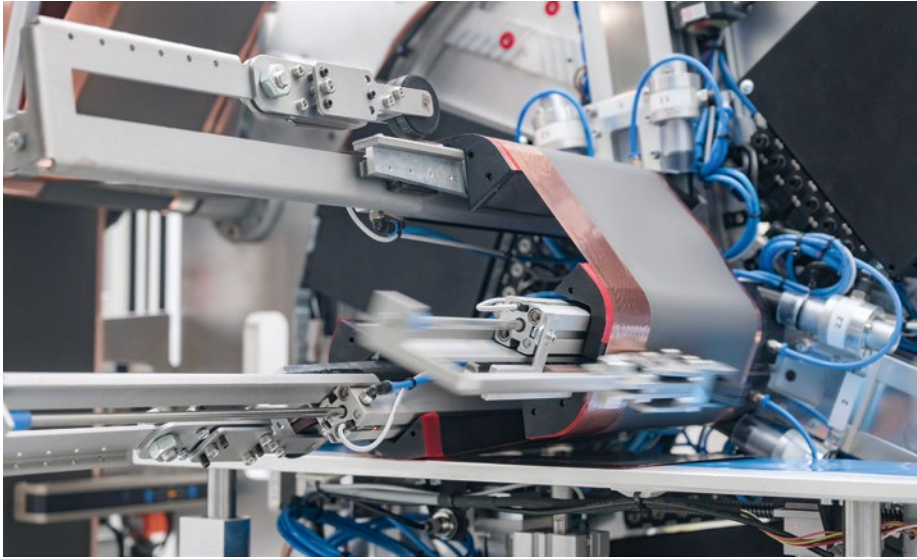
The material web is guided perfectly by the handling elements and ideally placed on the carrier; highly accurate synchronisation is ensured with the aid of end-to-end automation
