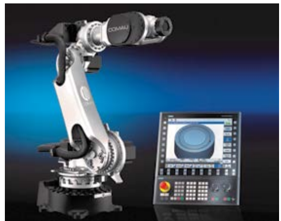
The project involves the complete integration of the robot arm from Comau in Siemens' Sinumerik system environment, which is made possible by the technological partnership between Comau and Siemens (source: Comau).
