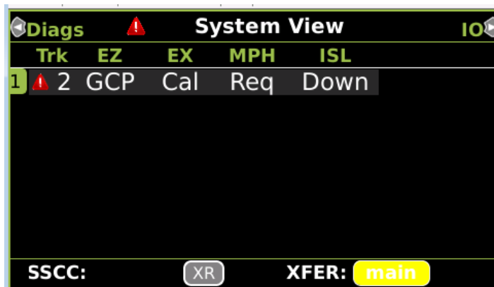
Figure 10 System Screen for GCP 4000 Transfer Extended
