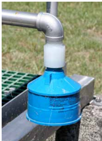
Ultrasonic transducers have a self-cleaning face, which literally shakes itself clean of dirt and buildup.
