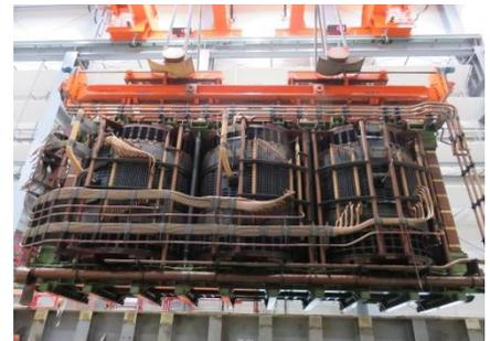
The dimensions of the unit are enormous, and a weight of 360 t meant a logistical challenge for everyone involved. The picture shows the active part is being removed from the tank.
