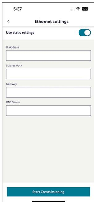
3. If you are configuring with static settings, enter the IP address, subnet mask, gateway, and DNS server details and tap on *Start Commissioning*.
