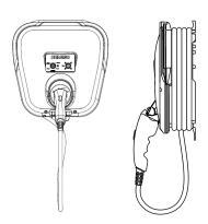
14.5" W x 16.0" H x 6.5" D (front of unit excluding connector) 15" minimum clearance recommended for connector when inserted
