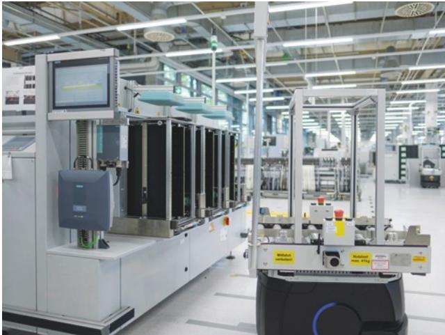
A core concept in the Karlsruhe manufacturing strategy is the use of automated guided vehicles (AGVs) for the material flow in the plant.
