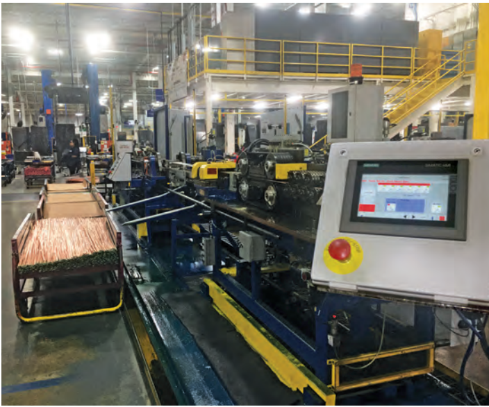
Figure 1. Left, view inside the Carrier factory coilshop, with newly installed Siemens SIMATIC Comfort Panel HMI in right foreground. Right, bent copper tubing destined for the insides of 1.5–5.0-ton residential air conditioners manufactured at the plant.
