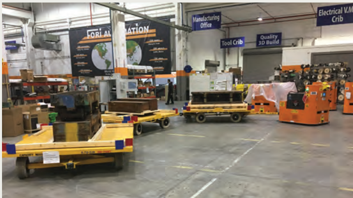
Fori Automated Tuggers capable of transporting up to 35,000 lbs. improve safety and ensure on-time delivery.
