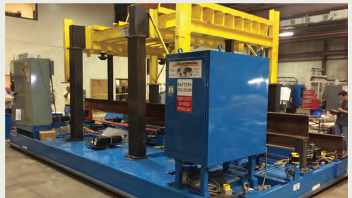
Fori Automation's automated guided vehicle (AGV) for transporting "drill & fill" tooling in manufacturing large commercial aircraft.
