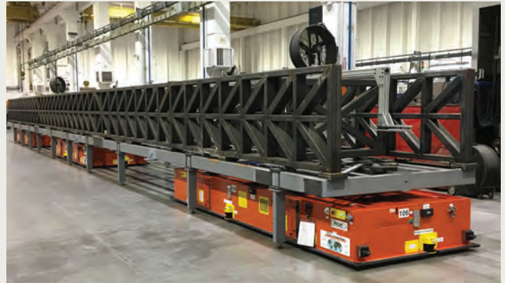
Synchronization of multiple vehicles for large Aerospace tooling transport increases flexibility, allowing various lengths and styles of tooling to be transported by a single vehicle design.
