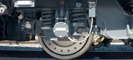
The propulsion unit consists of a pinion hollow shaft drive with the traction motor mounted directly to the truck frame by rubber elements. The gear is axle mounted riding on the wheel set with the other side mounted to the motor case by a reaction rod.
