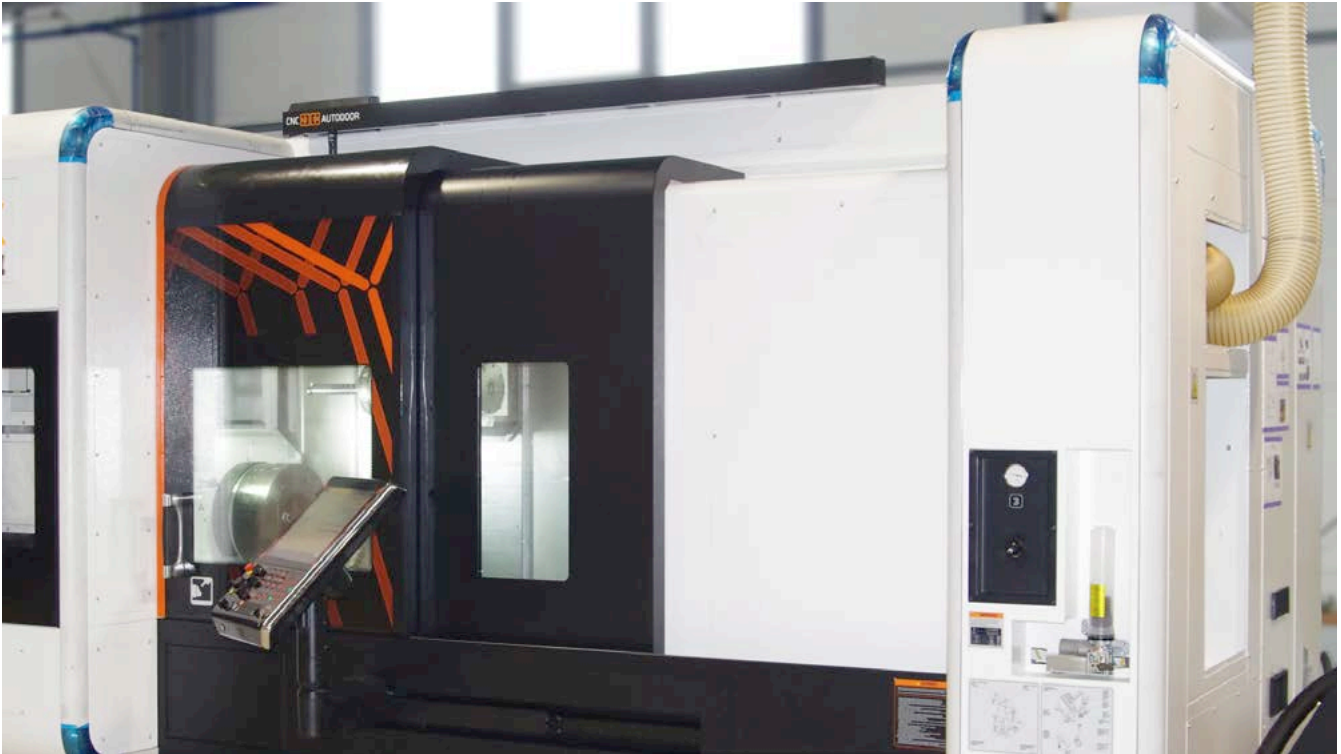
Example of the space-saving installation of the CNC AutoDoor drive rail
