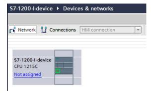
4. Double-click the IO device and configure all required modules and submodules.
