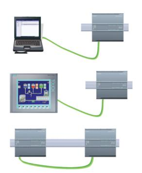
Programming device connected to the CPU
