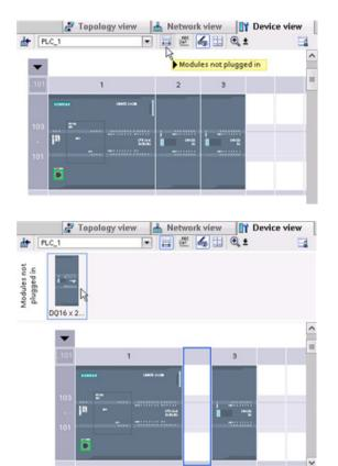
STEP 7 provides a storage area for "unplugged" modules. You can drag a module from the rack to save the configuration of that module. These unplugged modules are saved with your project, allowing you to reinsert the module in the future without having to reconfigure the parameters.
