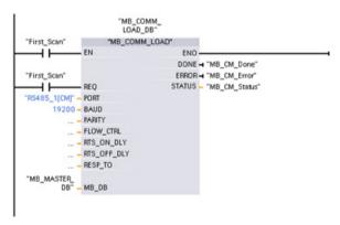
One MB\_MASTER instruction is used in the program cycle OB to communicate with a single slave. Additional MB\_MASTER instructions can be used in the program cycle OB to communicate with other slaves, or one MB\_MASTER FB could be re-used to communicate with additional slaves.
