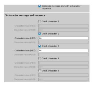
In this case, the end condition is satisfied when two consecutive 0x6A characters are received, followed by any two characters. The character preceding the 0x6A 0x6A pattern is not part of the end character sequence. Two characters following the 0x6A 0x6A pattern are required to terminate the end character sequence. The values received at character positions 4 and 5 are irrelevant, but they must be received to satisfy the end condition.
