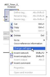
STEP 7 allows you to easily create or change the association of a DB for an instruction or an FB that is in an FB.
