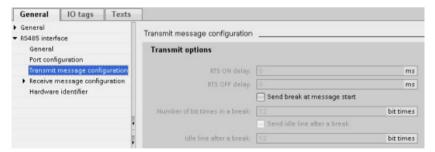
You can also dynamically configure or change the transmit message parameters from the user program by using the Send\_Config (Page 882) instruction.
