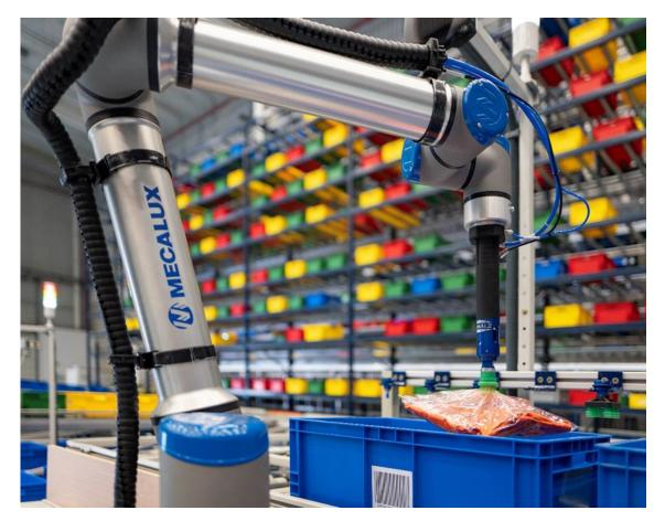
Simatic Robot Pick Al 3D vision software enables robots to pick any item in warehouse picking tasks, regardless of shape and size.
