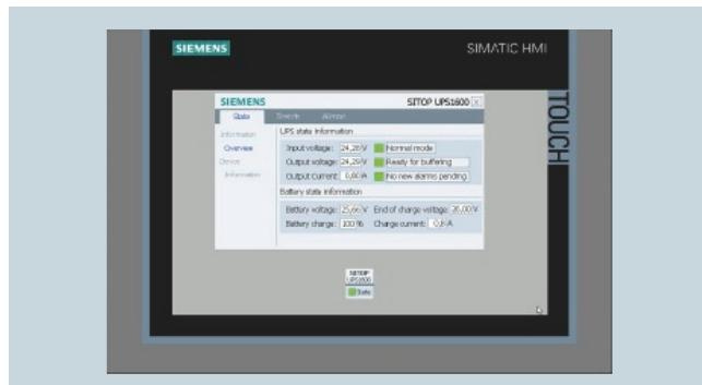
Diagnostics in WinCC: Prefabricated SITOP UPS1600 faceplates make visualization possible without the need for complicated programming.
