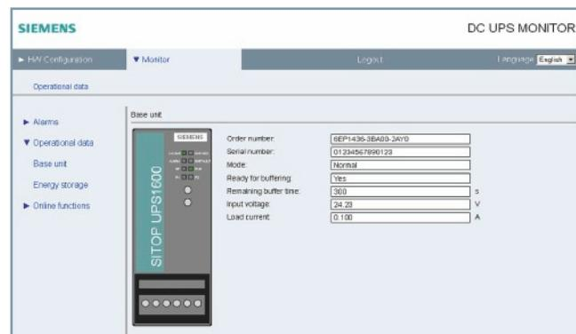
Remote monitoring: The integrated web server provides access to all relevant data of the uninterruptible power supply.
