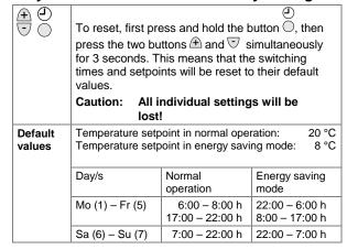
To reset, first press and hold the button O, then press the two
