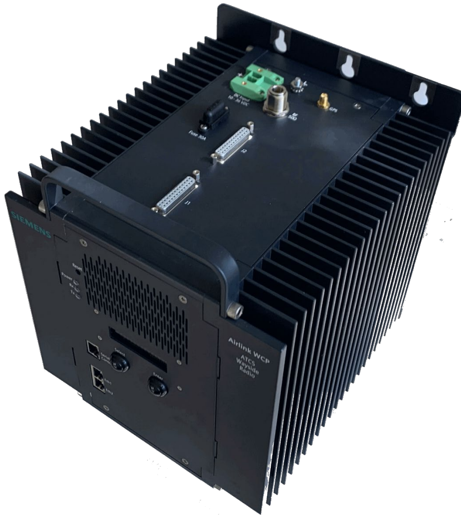
Figure 1-2 Airlink Wayside Communications Package (WCP) – Top/Right Side View
