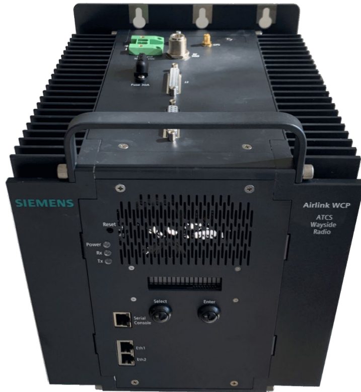
Figure 1-1 Airlink Wayside Communications Package (WCP) – Front/Top View
