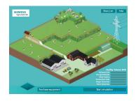
The farm is therefore a producer as well as a consumer; it can function either independently of the National Grid or as part of it. If the latter it can sell electricity to the grid as well as buying from it. After the system is set up it then runs for a period of time and performance data is produced. This shows whether a continuous supply was maintained, what the overall cost of running the system was and what the impact on the environment was. Changes can be made to improve performance.
