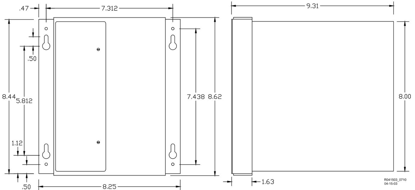
**Figure 3-3 Bidirectional Simulation Coupler Assembly Mounting Dimensions**
