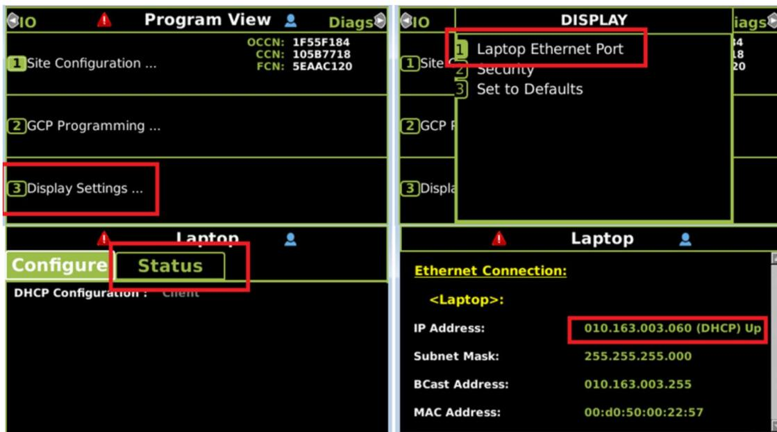
Figure 4-126 Finding IP Client Address
