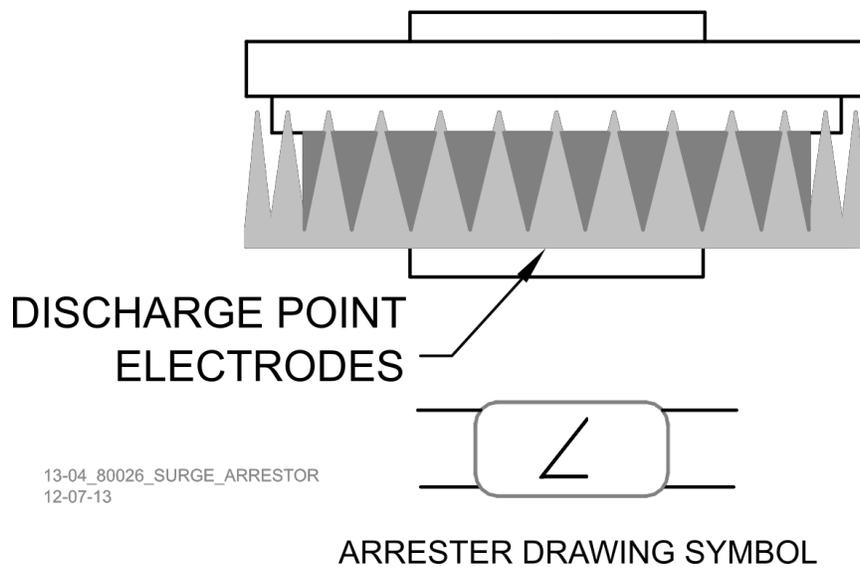
**Figure 3-4 Typical 80026 Surge Panel Arrester Mounting Position**
