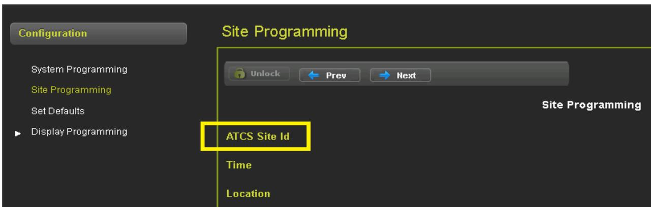
**Figure 6-11 Setting ATCS Address on WebUI**
