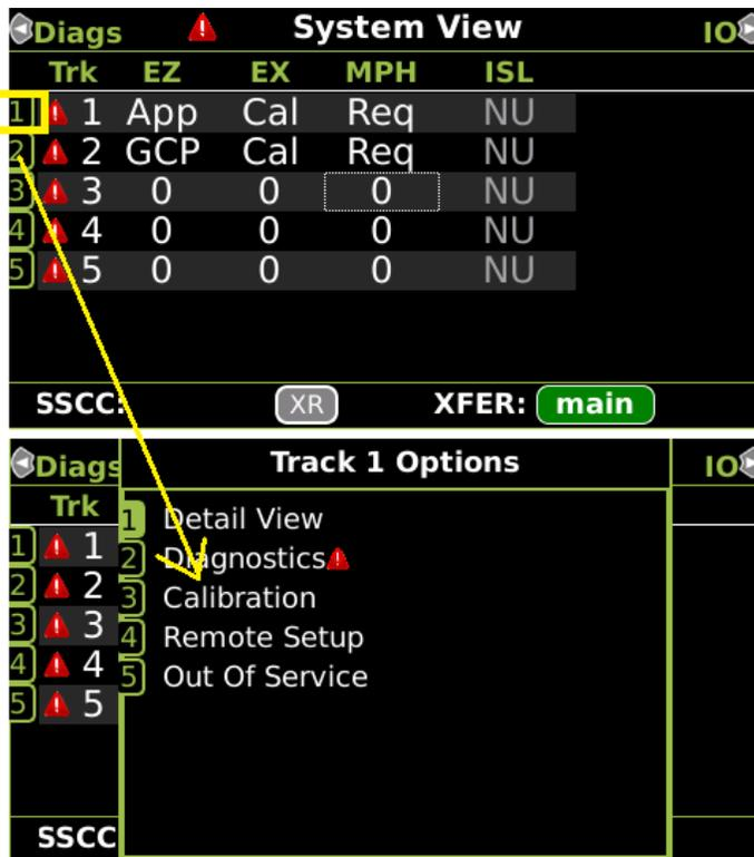
**Figure 6-2 Opening the Calibration Window**
