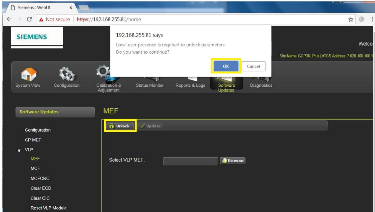
Figure 4-75 WebUI, GCP Menu – VLP MCF UNLOCK
