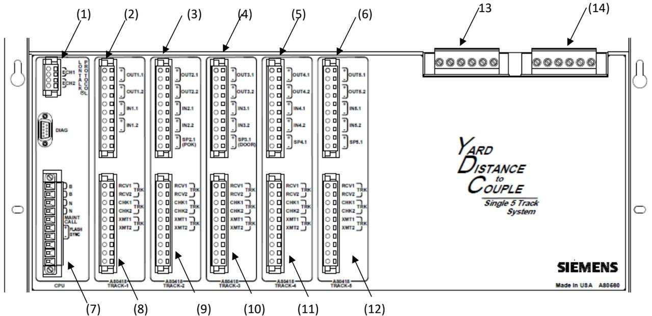
Figure 2-4 External Wiring Connectors
