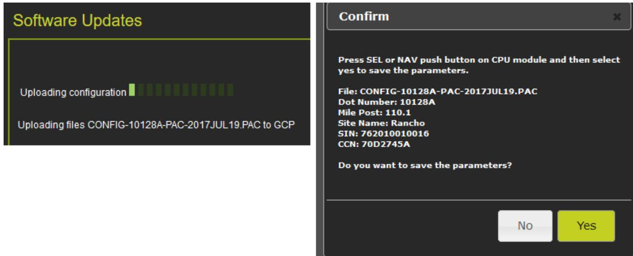
Figure 4-113 WebUI: Configuration Upload Progress and Final Check
