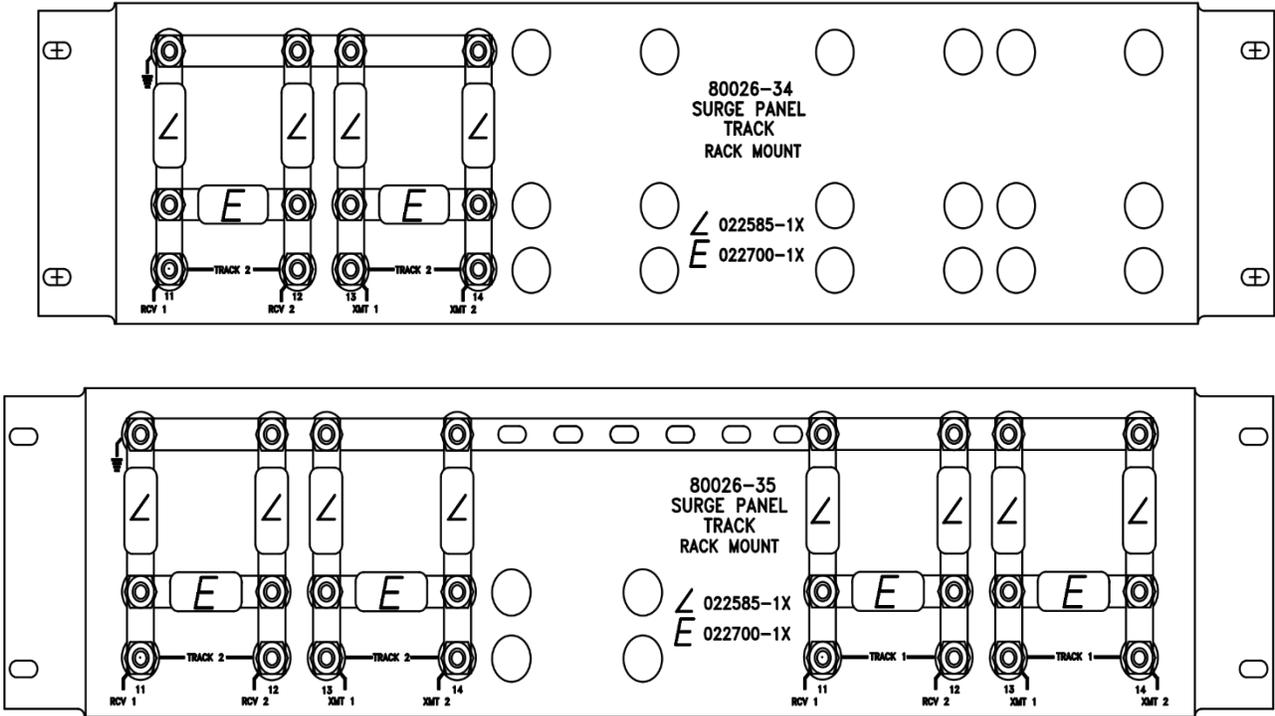
Figure 3-7 Rack Mounted Surge Panels, 80026-34 and -35
