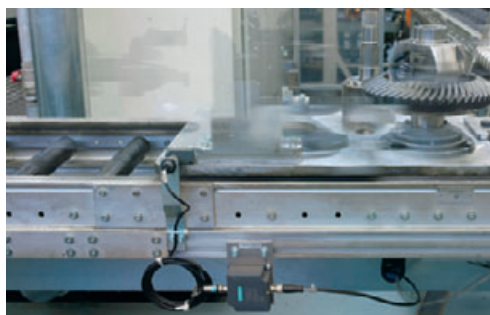
Simatic RF350R reader record the information of the RFID transponder on the pallets
