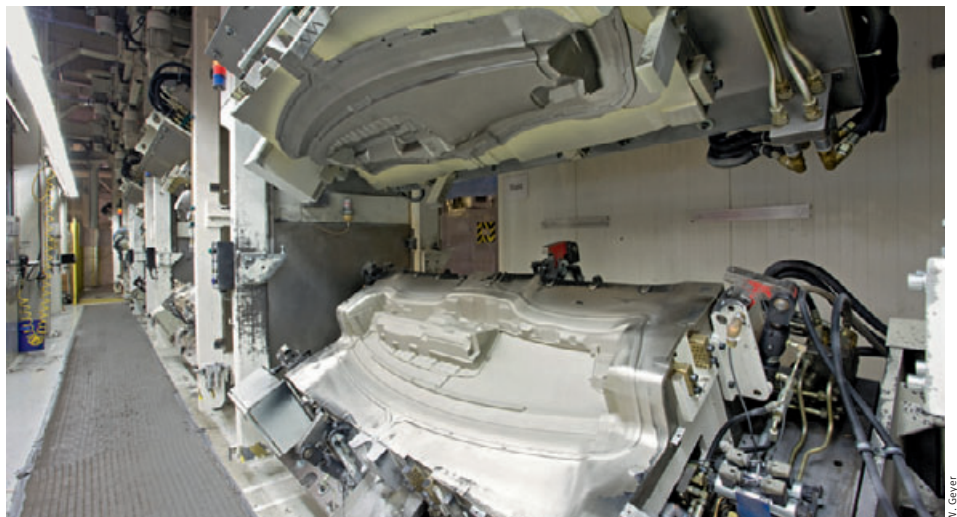
The mold carrier cars are transported via a 2-rail suspension track through the multistage casting process
