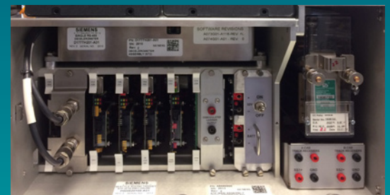
ATC Unit (Assembly No. NYK:P000620100-A01)
