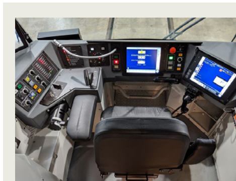
Light Rail Operator's Cab Console. ADU is left of center screen.
