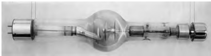
A Pantix rotating anode tube, 1933
