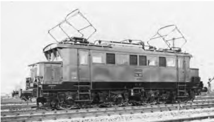
Passenger and freight electric locomotive E 44, 1933
