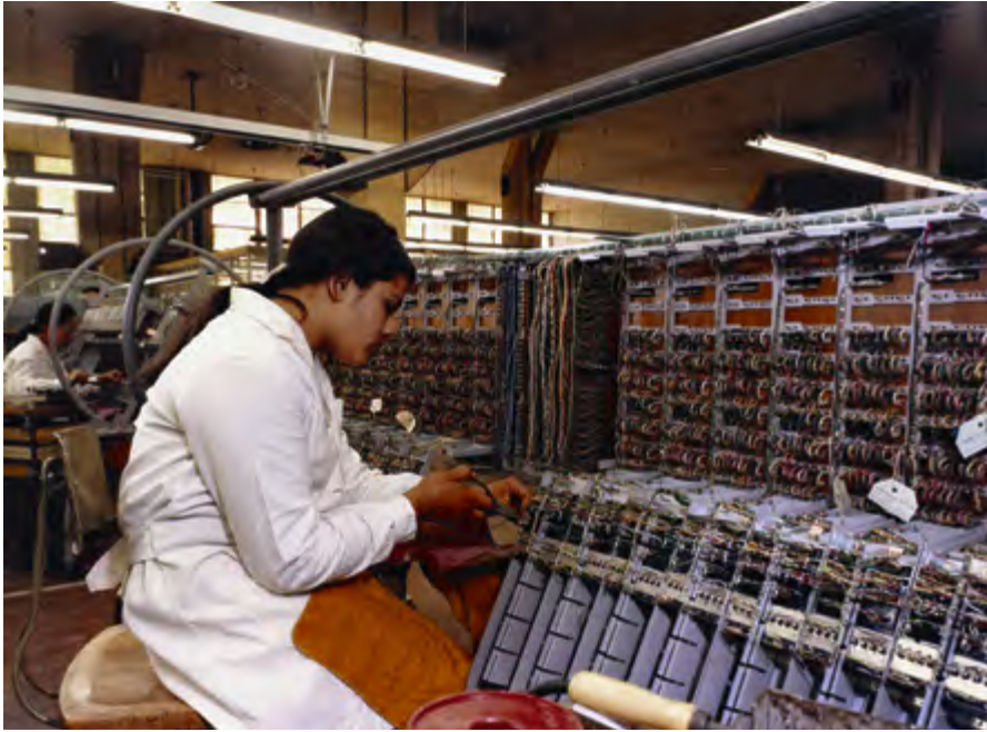
Wiring of telephone systems in the Siemens Ruta 8 factory in Buenos Aires, 1966
