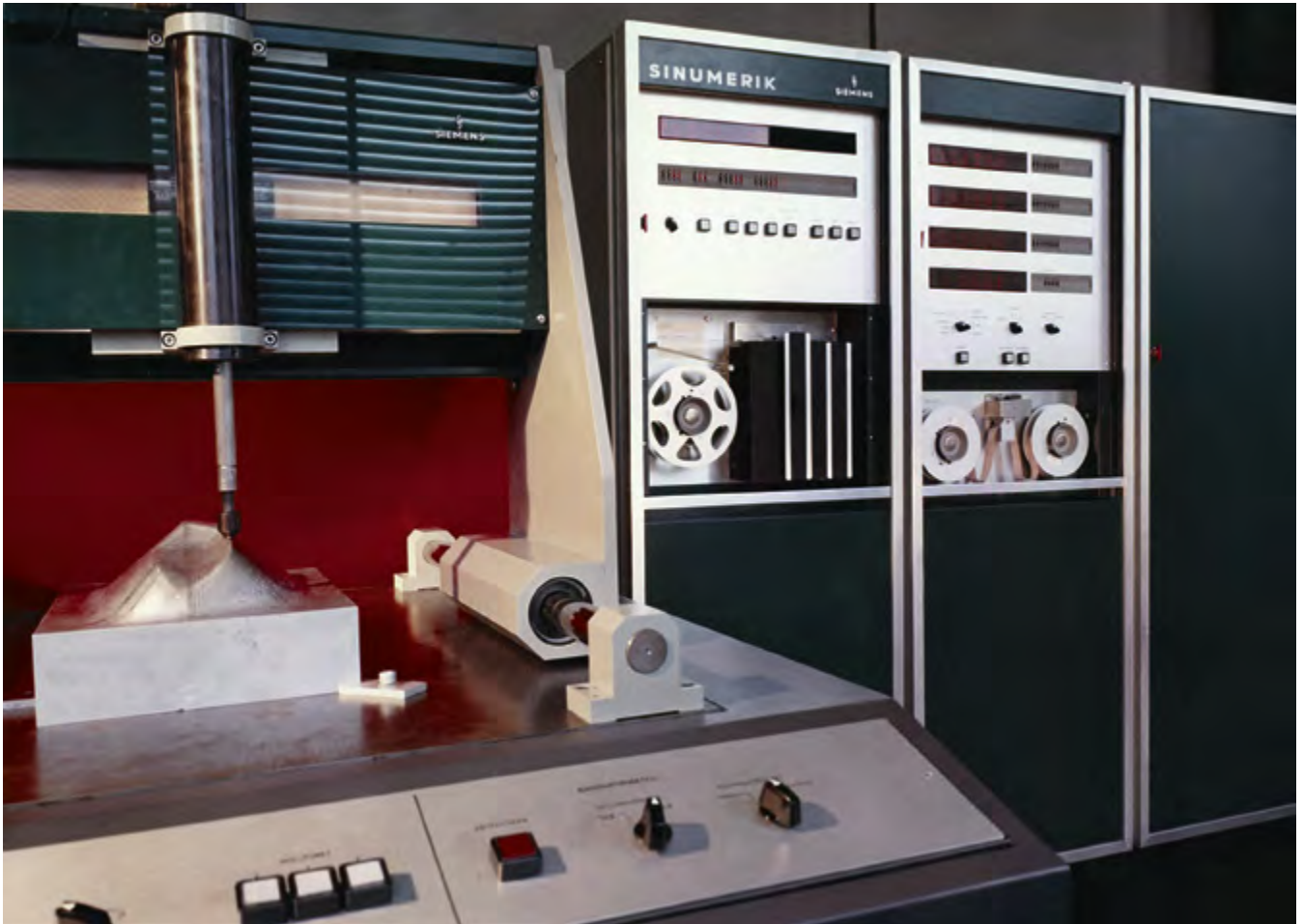
A milling machine with the SINUMERIK electronic control system, 1967
