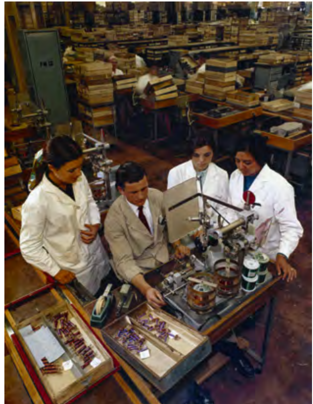
Coil winding in the Siemens factory Ruta 8 in Buenos Aires, 1966
