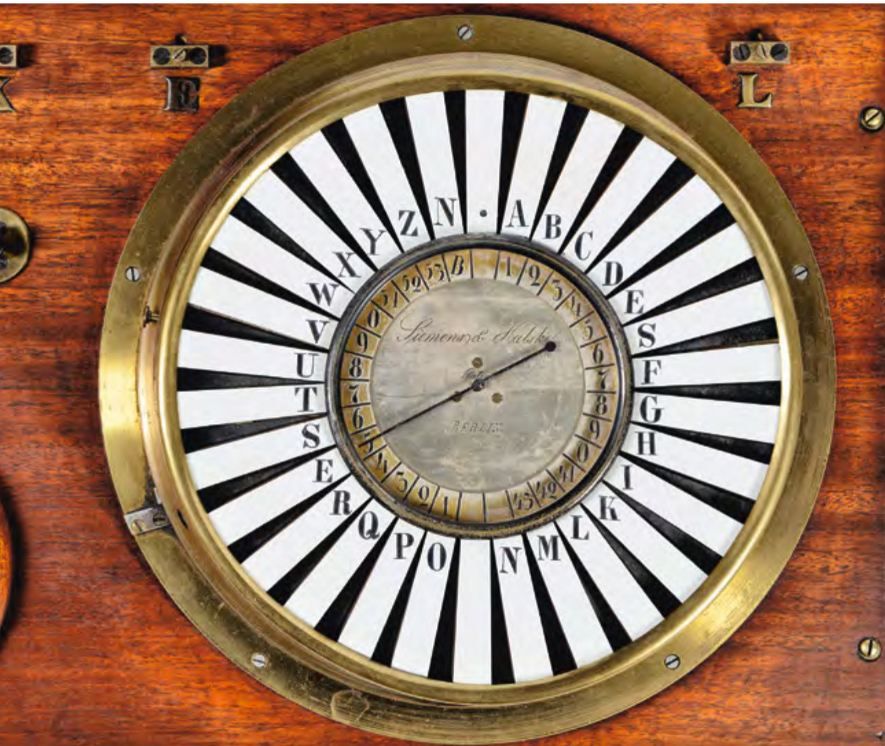
Werner von Siemens' electric pointer telegraph of 1847 (replica)
