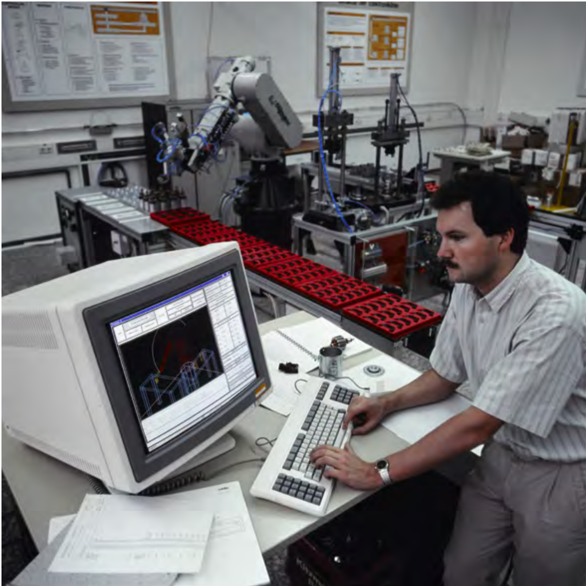
Experimenting with simulation software at Siemens for controlling a robot arm, 1987
