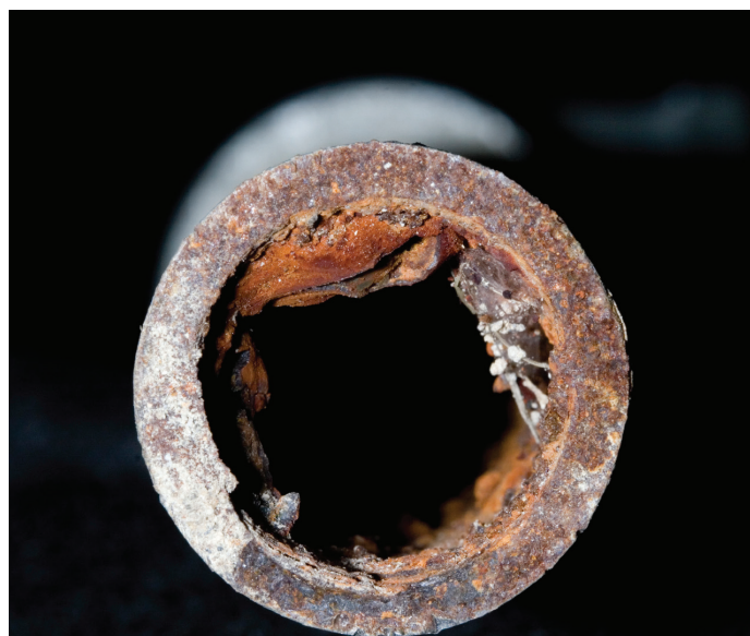
Debris and corrosion can cause system failure.
