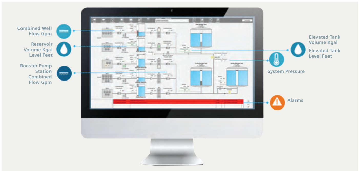
SIMATIC WinCC Open Architecture (OA) SCADA software provides an operational dashboard with system-wide visibility that the City of Hobbs never had before.
