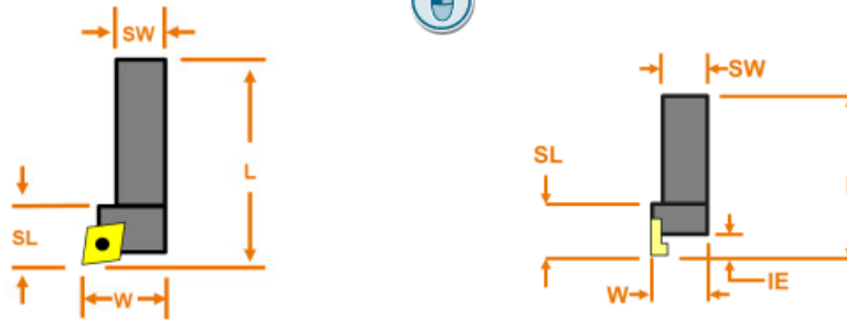
Figure 9-16 Parameters of a shank using the example of a turning tool and cutting tool
