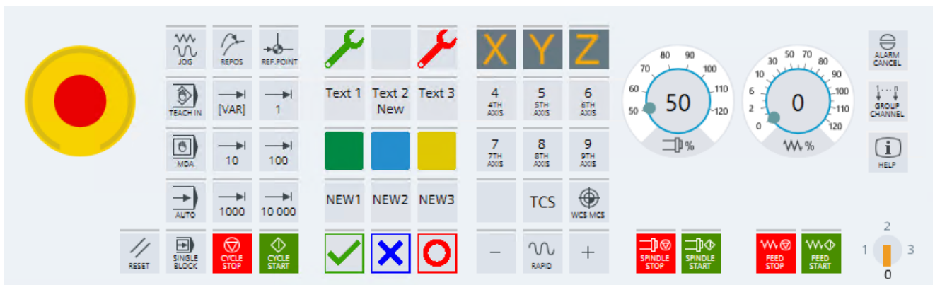
Figure 5-8 "User MCP" customer control panel
