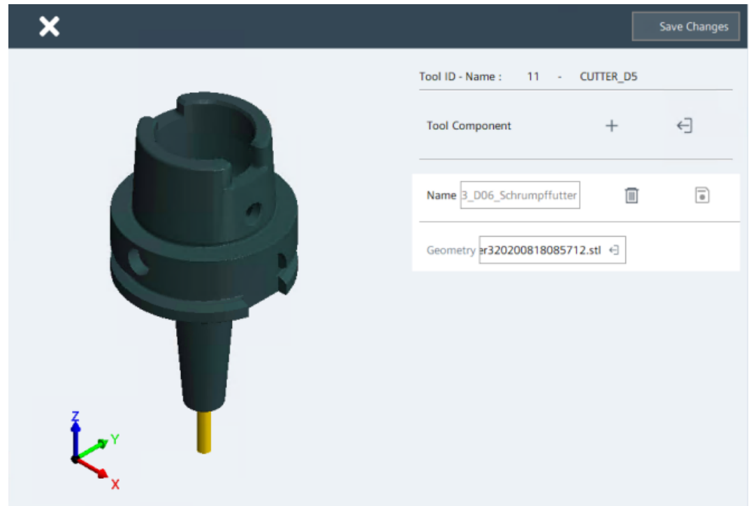
Figure 9-24 Tool holder from the library assigned to the tool
