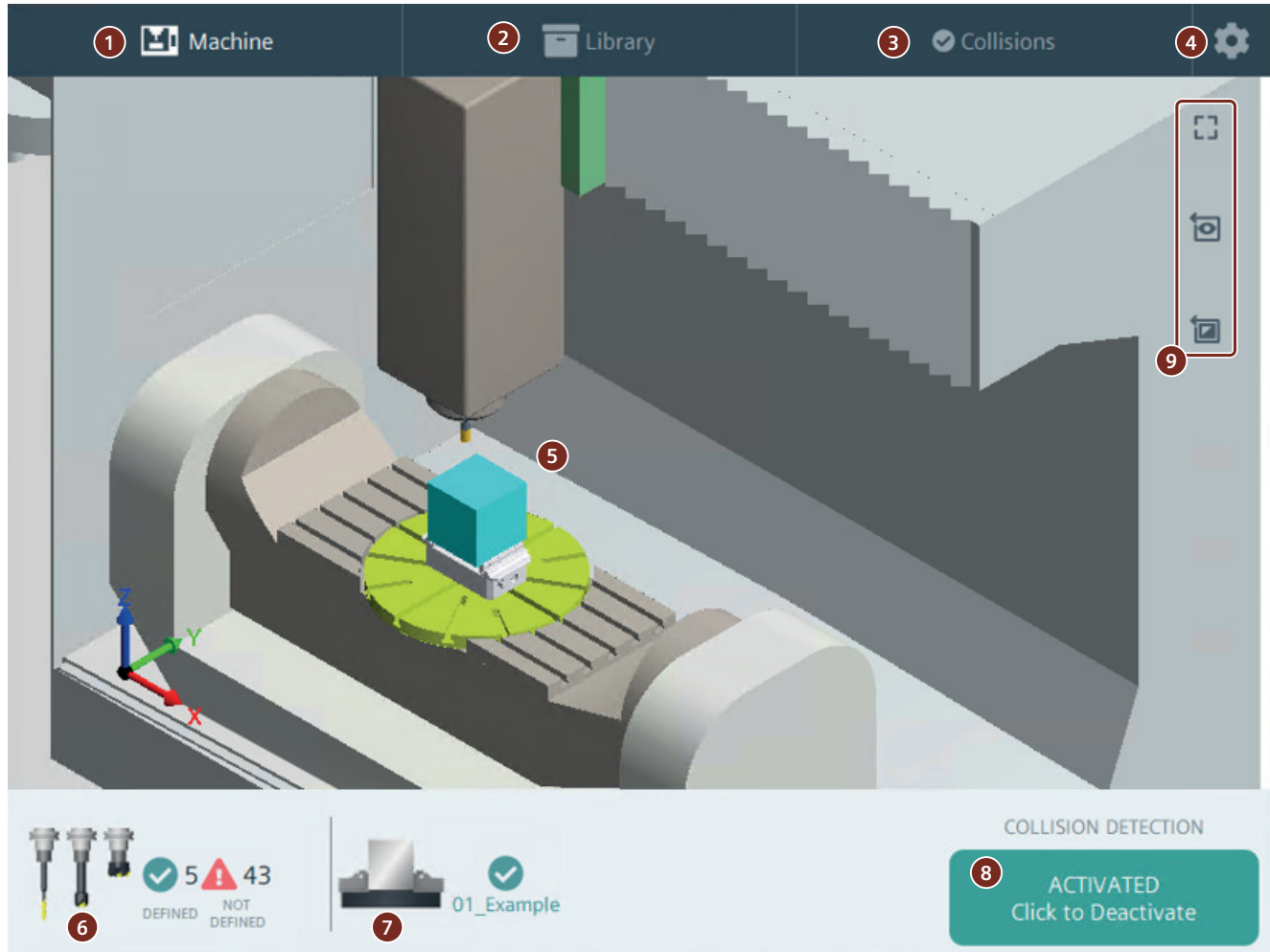
Figure 9-1 3D simulation, operating areas and functions using the example of a milling machine
