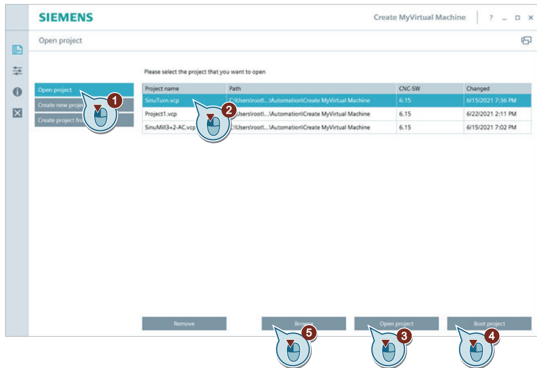
Figure 5-6 Open a project in Create MyVirtual Machine
