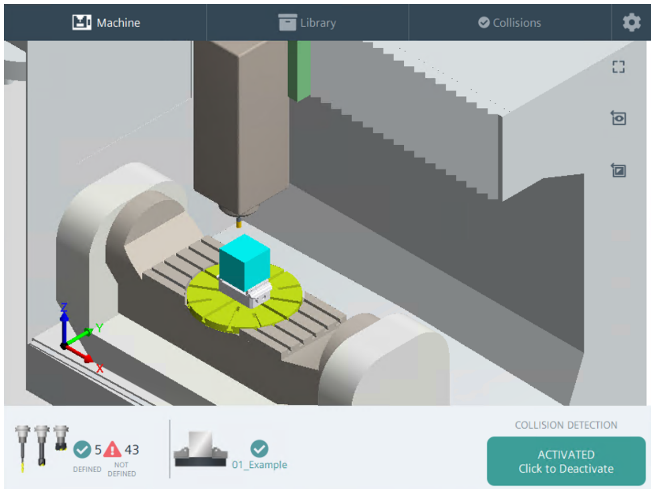
Figure 4-3 3D simulation in Create MyVirtual Machine
