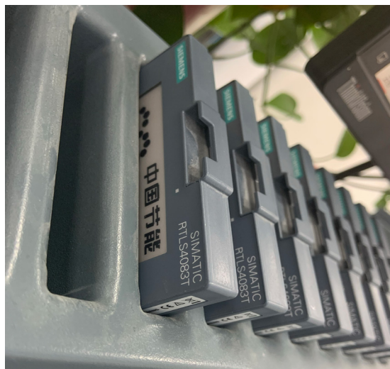
The real-time locating system SIMATIC RTLS enables personnel locating in underground sewage treatment plants.
