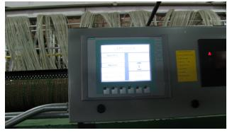
**Description of Application:** Application allows any maintenance personal to walk up to the machine and be able to troubleshoot if the machine is down electrically. The HMI will display what's holding the machine out. On the monitoring side of the application you can keep up with each machines' efficiency and look at all your different downtime codes.
