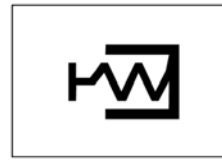
Fig. 193: "Closing spring not charged" indication
