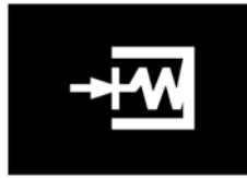
Fig. 192: "Closing spring charged" indication
