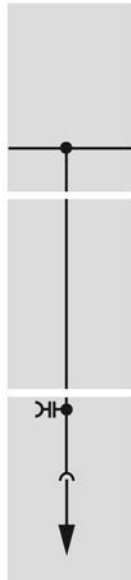
Cable connection panel
