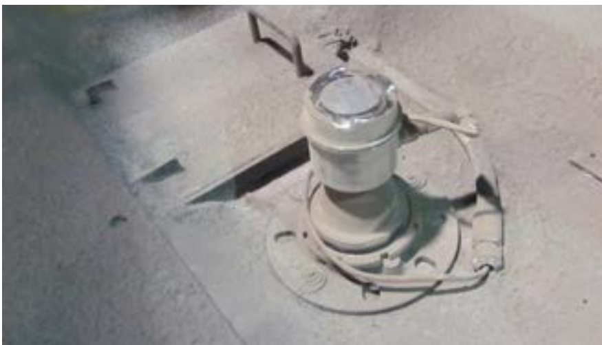
Fig. 2: The Sitrans LR560 is the ideal radar device for dusty environments. In addition, it emits a short wavelength (78 GHz), so is able to accurately measure the level of solids, even when the material is piled on a steep angle.
