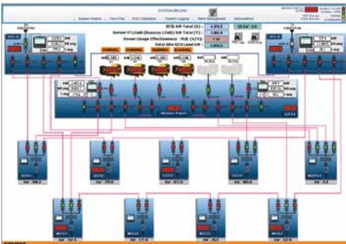
Example screen from WinPM.Net software showing electrical system diagram with multiple real-time metering points
