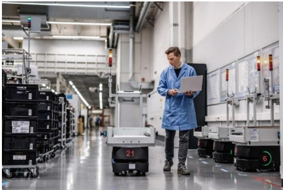
Automated guided vehicles optimize material flow and logistics across the factory floor
