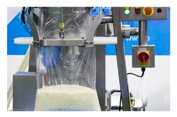
**4. Higher yield** – SIWAREX scale electronics provide high accuracy, even in demanding applications, with measurement rates up to 1000 measurements per second. And by plugging the scale electronics directly into the IO of the control system, weight measurements are communicated on the high-speed bus between the IO and the control system. This allows high-speed machines such as filling processes or batching systems to operate at maximum speed, increasing efficiency and throughput.
