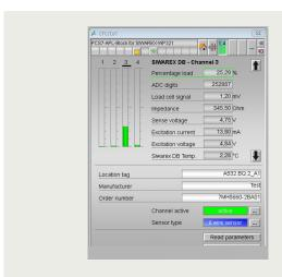
**3. Improved product quality –** SIWAREX scale electronics have onboard diagnostics to detect a problem with the load cells, and with the add-on APL library, these diagnostics are reported on the operator station. If a problem is detected, the operator is alerted and can take immediate action to ensure product quality is not affected. When used with the SIWAREX
