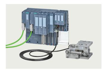
**1. Reduced downtime** – SIWAREX scale electronics plug directly into the IO of the control system. With the PCS 7 control system's add-on Advanced Process Library, the function blocks and faceplates are prebuilt to allow full integration of the weighing system in just a few minutes.
