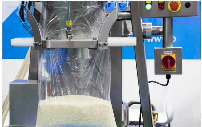
**4. Higher yield** – SIWAREX scale electronics provide high accuracy, even in demanding applications, with measurement rates up to 1000 measurements per second. And by plugging the scale electronics directly into the IO of the control system, weight measurements are communicated on the high-speed bus between the IO and the control system. This allows high-speed machines such as filling processes or batching systems to operate at maximum speed, increasing efficiency and throughput.
