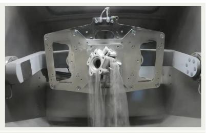
Additive Manufacturing and CNC in one software - CNC controlled removal of support structures
